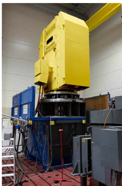
Caption: Menzel Elektromotoren now also performs load tests on large industrial motors in a vertical installation position
