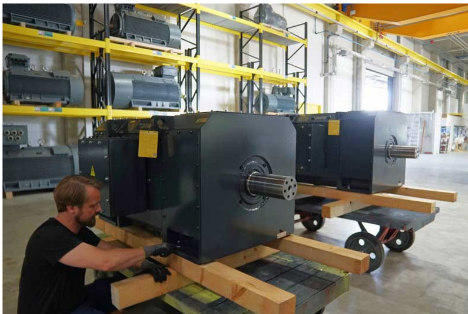
Caption: Two identical DC motors on the way to driving a rolling mill
