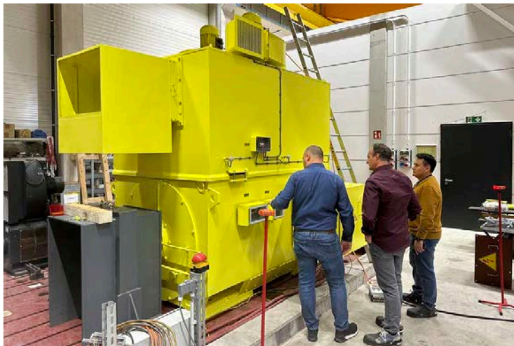
Caption: Menzel Elektromotoren thoroughly tests all motors before shipping; pictured: test engineer, sales partner and customer with the new mill motor in the load test field
