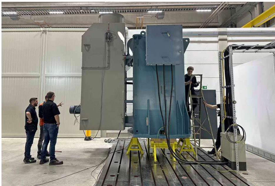
Caption: Menzel Elektromotoren has manufactured its largest low-voltage motor to date: a 20-ton pump motor
