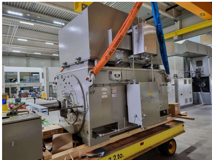
Caption: Menzel quickly configures squirrel cage motors in ignition protection type Ex p pressurization in device categories 2G and 3G in a wide output range from stock
