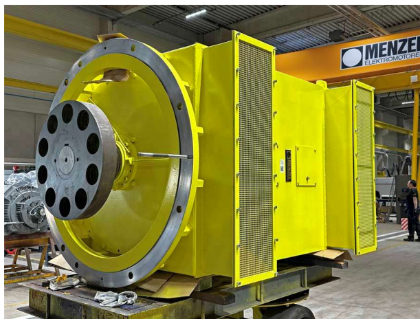
Caption: Menzel has tailored a squirrel cage motor based on its modular motor range, creating a one-to-one replacement for a 50-year-old pump motor in a combined heat and power plant
