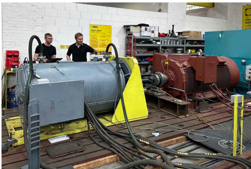
Caption: Menzel thoroughly tested the ship motors in its inhouse test field (here: squirrel-cage motor with water jacket cooling)
