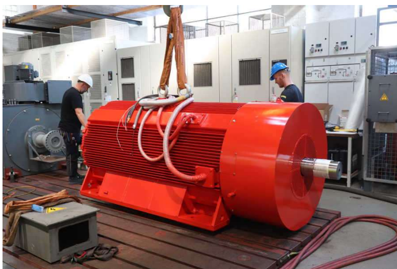
Caption: Menzel has tailored three-phase squirrel cage motors in frame size 630 for installation inside pit fans, including the manufacture of bespoke casings with cooling fins
