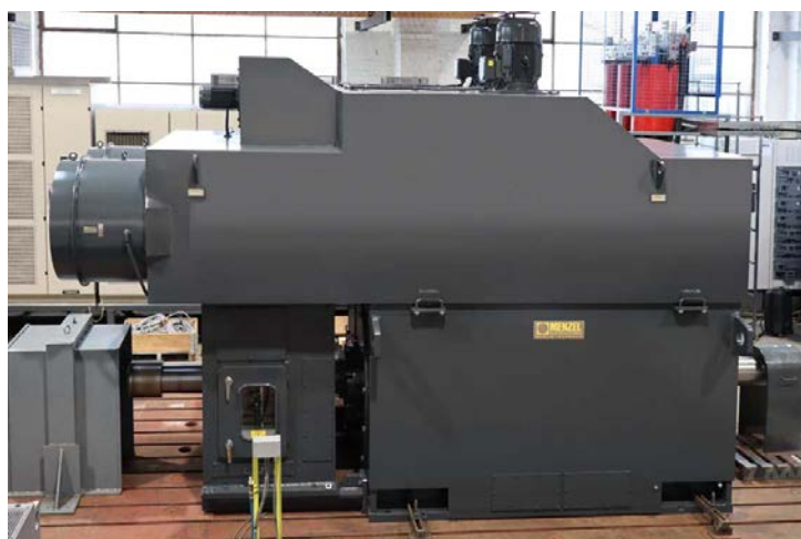
Caption: The custom-made slip ring motor with two shaft ends can replace two different mill motors as well as a fan motor – this saves money and space in spare parts management
