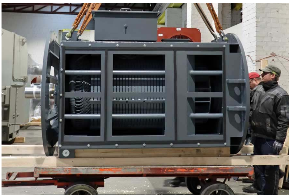
Caption: The flexibly designed spare can replace either of four beet pulp dryer motors in various sugar plants
