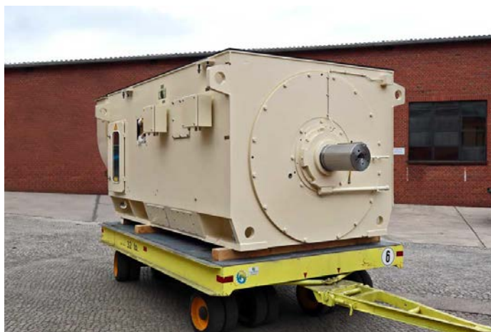
Caption: German motor manufacturer Menzel adapted the slip ring motor from its modular MEBSSL series to customer specifications at short notice
