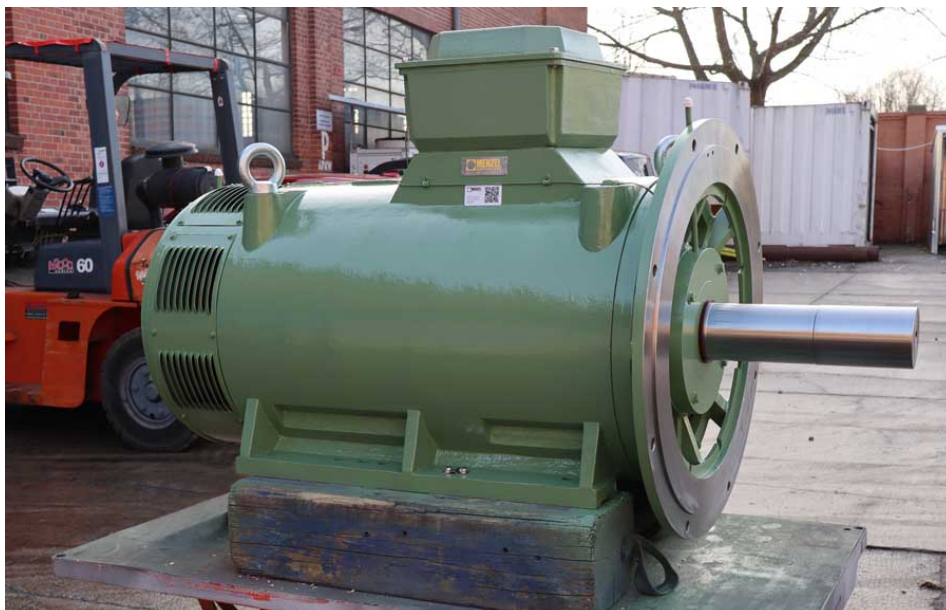
Caption: Menzel built the generator with a special shaft to withstand the large radial forces in the Pelton wheel application
