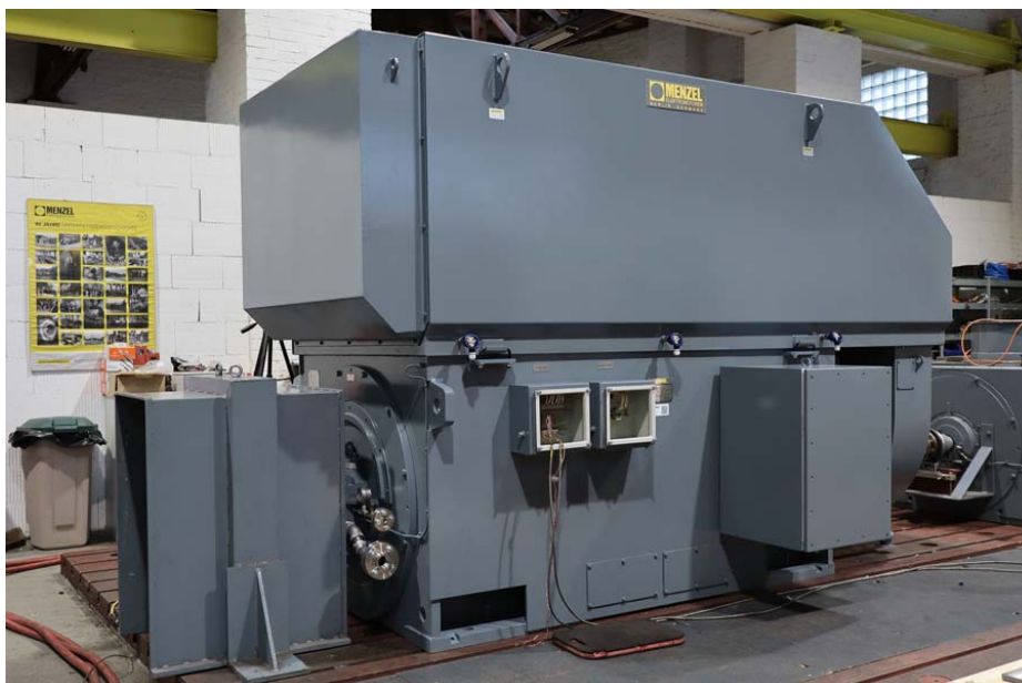
Caption: Menzel adapted the motors to the electrical and mechanical requirements and finally tested them in the in-house test field
