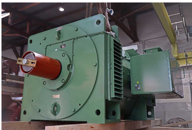
Caption: Menzel modeled the DC motor on an old roller motor, configuring it so it can replace either this motor or a coiler drive in the same rolling mill if necessary
