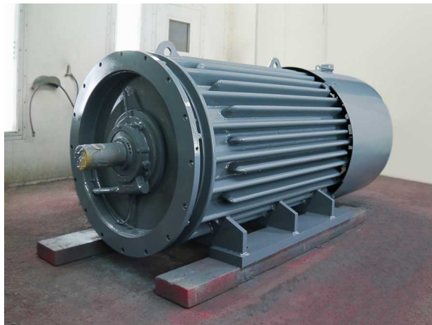
Caption: Menzel's large motor inventory includes unusual configurations such as this 12-pole medium-power motor
