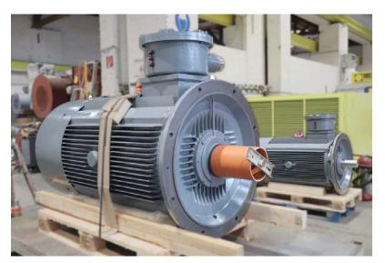
Caption: Menzel stocks up on components to enable faster delivery of IP67 motors – the picture shows two motors for a pump station in Egypt
