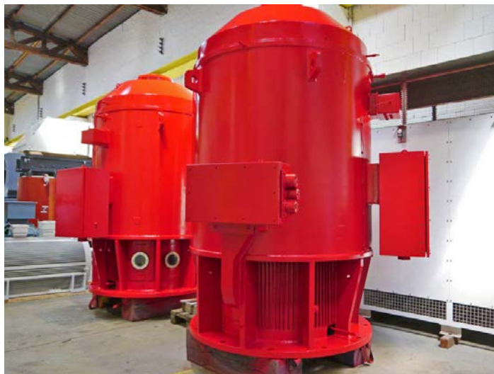
Caption: Menzel Elektromotoren builds vertical motors to measure – including hand-welded motor housings for efficient cooling
