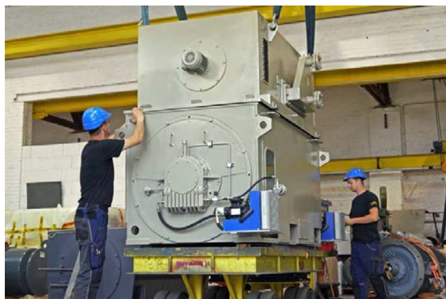
Caption: The water-cooled motor for driving a reciprocating compressor withstands high ambient temperatures
