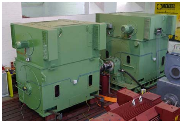
Illustration: The drive system for transformer inspections was manufactured and tested under load in Berlin
