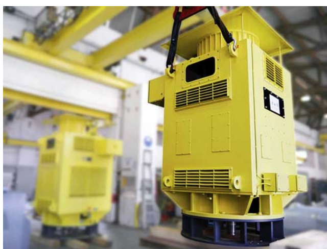
Illustration: Menzel manufactured and load-tested customized replacement motors for a waterworks
