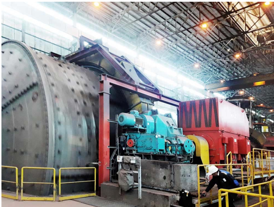
Illustration: The configuration for a ball mill that crushes rocks required a very robust drive that withstands dust and vibrations
