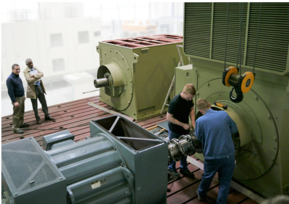
Illustration: Berlin-based Menzel Elektromotoren operate two in-house load test fields inside a state-of-the-art facility
