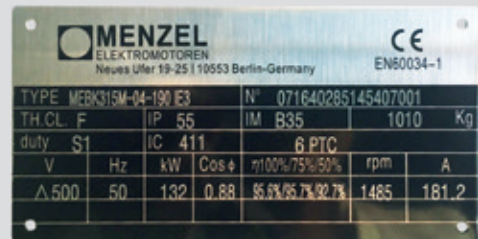
Figure: Identification of the energy efficiency class on a MENZEL motor identification plate
